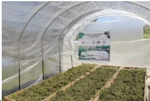
Figure 2. Plastic house-type solar dryer (Carlos Bertello, GIZ EnDev Peru)
