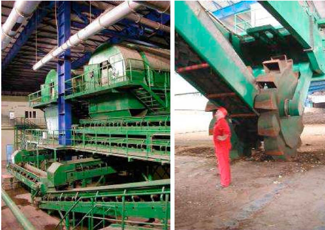
Fig. 53. MBT Istanbul: Mechanical pre-treatment (left), turning system in aerobic biological stabilization system (right)
